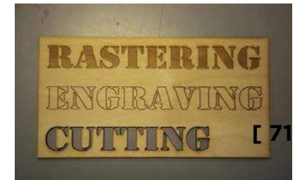
example of laser rastering, engraving and cutting
